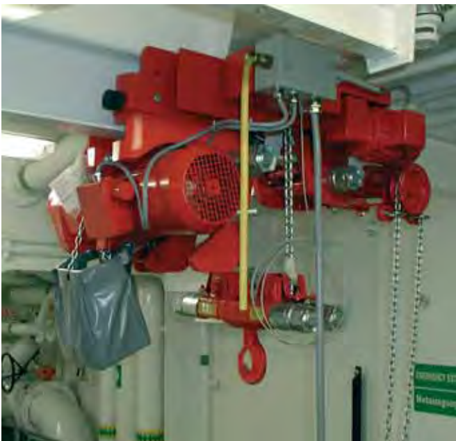
Electric Chain Hoist Type 29/06 EH ultralow headroom configuration with hand geared trolley capacity: 2 t
