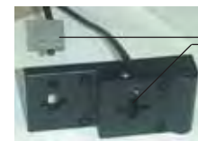
operational limit switch
