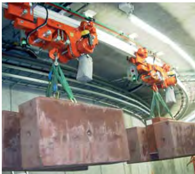
Electric Chain Hoist Type 29/06 EE ultralow headroom configuration with swivelling electric trolley capacity: 5 t
