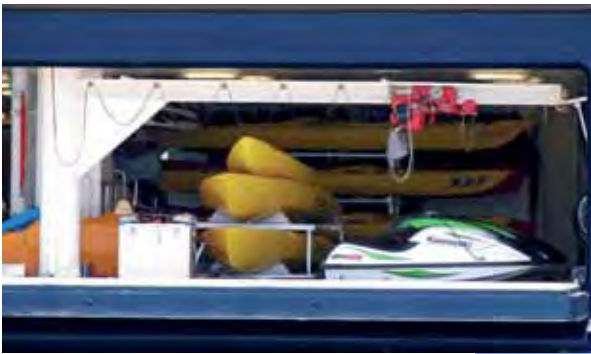
Jib Crane with Electric Chain Hoist ultralow headroom configuration and beam locking device
