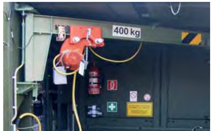
Wall-mounted Jib Crane Type 320/01 E with Electric Chain Hoist Type 28/06 ER with push travel trolley capacity: 400 kg
