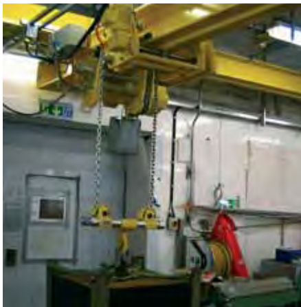
Single Girder Manual Underslung Crane Type EDHH with Spur Gear Hoist Type 29/98 HH rack and pinion drive capacity: 3 t
