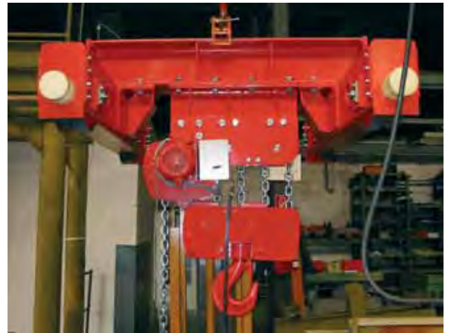
HADEF double-rail crab Type 35/04 with electric chain hoist Type 66/04 AK capacity: 25 t for Double Grider Electric Overhead Travelling Crane Type ZEE span: 15 m
