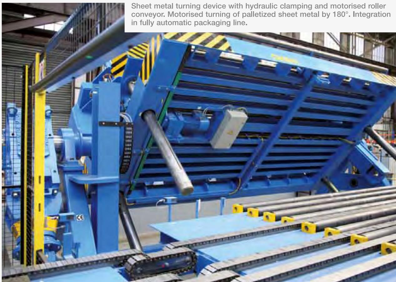
Sheet metal turning device with hydraulic clamping and motorised roller conveyor. Motorised turning of palletized sheet metal by 180°. Integration in fully automatic packaging line.
